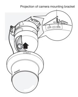
3 Turn this bracket clockwise until the projection of the camera mounting bracket aligns with "LOCK" of this bracket.
