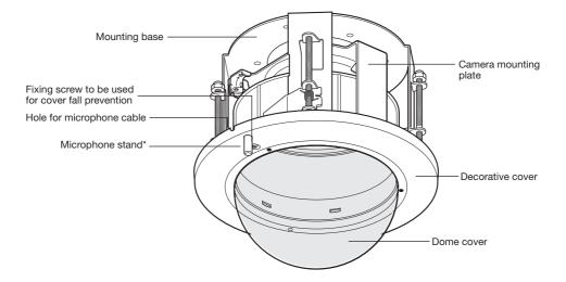
\* If a tiepin type microphone is used, mount the microphone on the rubber-made microphone stand. Unless the microphone is used, cut the rubber with a nipper or conduct another treatment.
