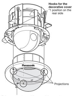
Fixing screw to be used for cover fall prevention
