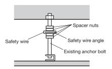
Connect the mounting base to another tip of the safety wire.
