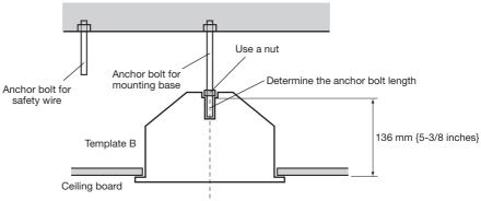
Install the anchor bolt in the center of the hole
