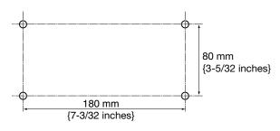
\* The above measurement diagram shows the view when standing on the floor and looking up at the ceiling.
