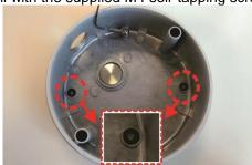
4. Loosen the cable clamp slightly. Remove the internal portion of the rubber plug from the cable entry hole of the wall mount junction box cover.
