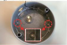
3. Place the supplied waterproof washers on the two screw holes. Match the two screw holes on the wall mount junction box with the plastic screw anchors (if used) at the installation location. Then, fasten the wall mount junction box to the wall with the supplied M4 self-tapping screws.
