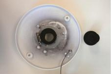
5. Thread the connectors of the All-In-One cable of the camera one-by-one through the cable entry hole.
