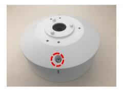
11. Align the two screw holes on the camera with the screw holes on the wall mount junction box cover and fasten the camera with the M4 machine screws. The drainage hole should point down when installing horizontally.
