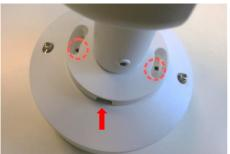
12. Rotate and point the camera to a desired direction and tighten the two set screws as shown below. The wall mount junction box installation is complete.
