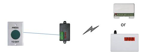
RTI10 universal 4-channel transmitter is designed to take any dry contacts as inputs from button/switch/relay devices, and transmit them to ACTIVOR receivers.
