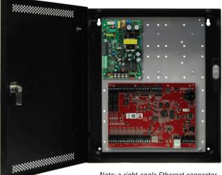
Note: a right-angle Ethernet connector is required when mounting an LP1502
