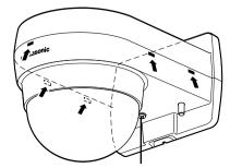
Fixing screw to be used for cover fall prevention
