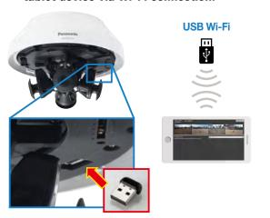
Insert USB Wi-Fi device\* to the USB terminal on multi-sensor camera
